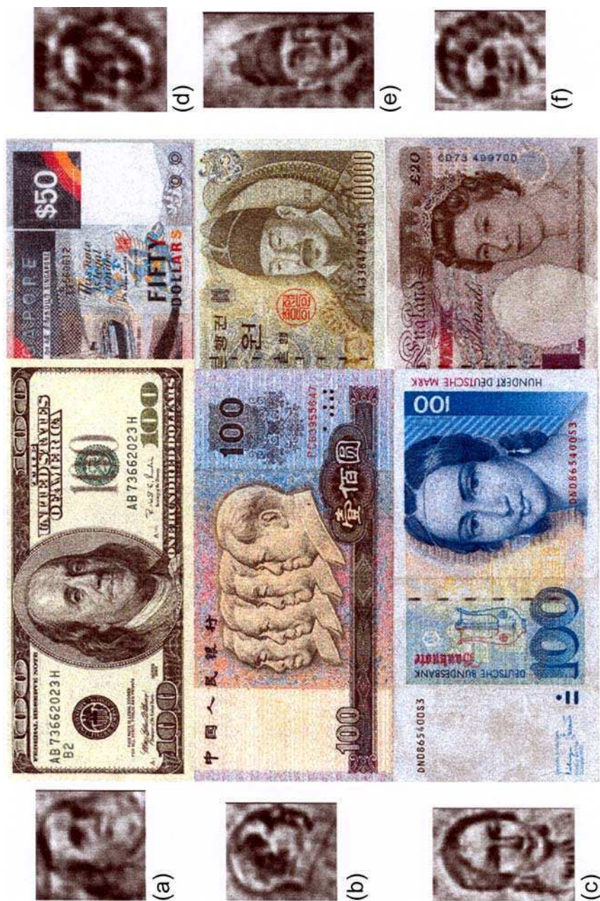
Figure 10 Terahertz wave images of the watermarks of several common bills: (a) 100 U.S. dollars; (b) 100 Chinese yuan; (c) 100 German marks; (d) 50 Singapore dollars; (e) 10,000 Korea won; (f) 20 British pounds.
